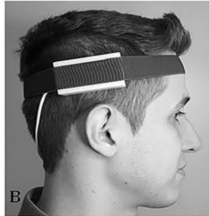
A , Braincare intracranial pressure (ICP) monitor 2000; B , Braincare ICP non-invasive sensor.
