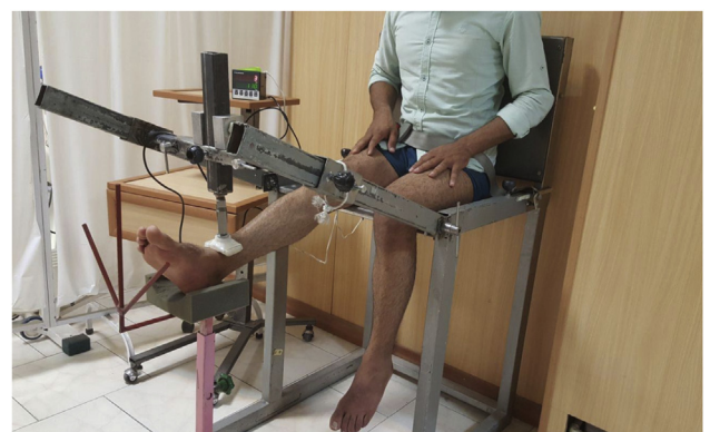
Fig. 1. The designed chair to measure the maximum SLR force.
